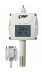
Ambient thermometer hygrometer barometer. Outdoor, indoor use. Built-in relative humidity, temperature, atmospheric pressure sensors. Measured values are also converted to other humidity interpretation: dew point temperature, absolute humidity, specific humidity, mixing ratio, specific enthalpy.
