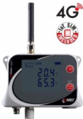
4G Datalogger is designed to record temperature from two external Pt1000 probes. In case of exceeded set limits, SMS and JSON messages can be sent via 4G data connection. Measured values can be sent to the internet storage [COMET Cloud](#), which is a complete monitoring, alarm and analysis system.
