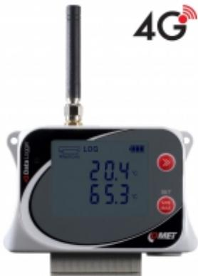
4G Datalogger is designed to record temperature from four external Pt1000 probes connected to the terminal board. In case of exceeded set limits, SMS and JSON messages can be sent via 4G data connection. Measured values can be sent to the internet storage [COMET Cloud](#), which is a complete monitoring, alarm and analysis system.
