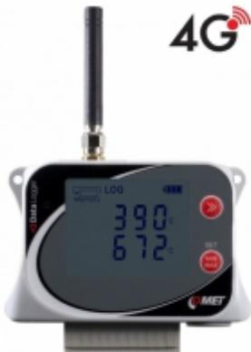
Datalogger is designed to record temperature from three thermocouples, one Pt1000 probe and one internal temperature sensor. In case of exceeded set limits, SMS and JSON messages can be sent via 4G data connection. Measured values can be sent to the internet storage [COMET Cloud](#), which is a complete monitoring, alarm and analysis system.
