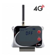
4G datalogger is designed to record from four binary inputs or from two pulse and two binary inputs. In case of exceeded set limits, SMS and JSON messages can be sent via 4G data connection. Measured values can be sent to the internet storage <a href="COMET Cloud">COMET Cloud</a>, which is a complete monitoring, alarm and analysis system.
