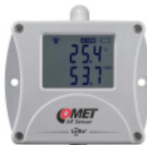
The W3911 sensor with LoRaWAN network output measures the temperature and humidity [from an external probe on the cable](#) and can be installed directly in the measured environment thanks to its IP65-rated enclosure. LoRa devices are powered by a replaceable battery with a lifespan of up to 10 years (3 years standard).
