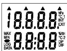
Connect the external probes to the connectors before switching ON the instrument. Switch ON the instrument by pressing ON/OFF key. After switching ON the instrument all symbols on the LCD are displayed. If the ON/OFF key is being held pressed, all LCD symbols are displayed till the key is released.
