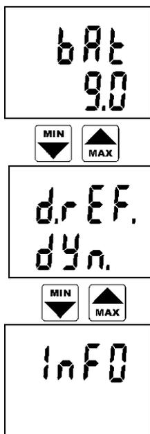
Battery voltage of partially loaded battery is displayed. This value illustrates battery condition.
