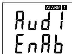
**Acoustic alarm assign to Relay2**
